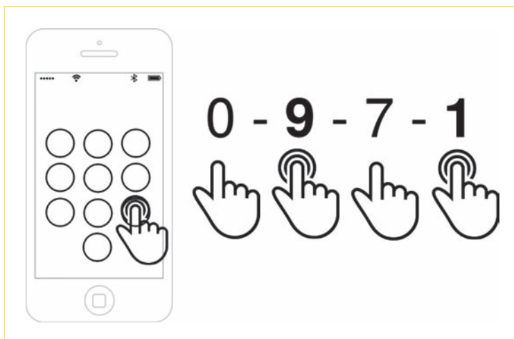
Figure 1. Schematic overview of force-PINs. Digits can either be entered with shallow or deep pressure (with vibration feedback) on a pressure-sensitive touchscreen.
