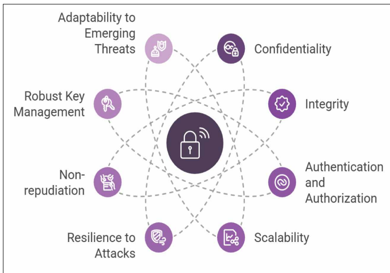
FIGURE 2. Illustration of key security requirements for a cryptographic scheme to secure IoT systems.
